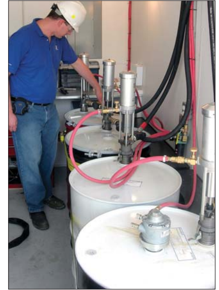
Prime and sealant components are dispensed automatically from drums.
