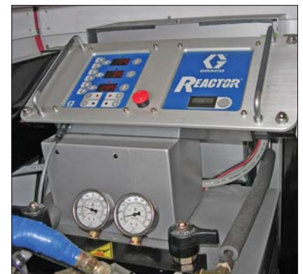
Material components are heated in a reactor before spraying.
