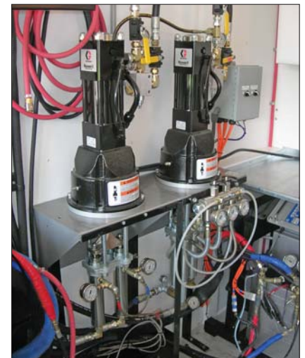
Proportioners deliver material in appropriate amounts.
